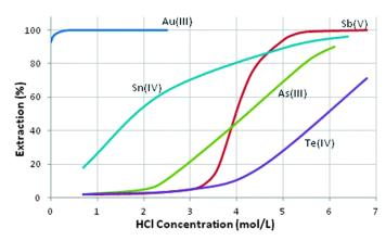
Fig. 10- Selectivity of gold extraction with dibutylcarbitol. 22
