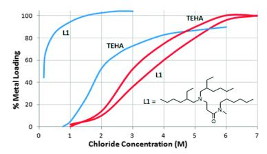
**Fig. 11** Loadings of [ZnCl<sub>4</sub>]<sup>2-</sup> (blue lines) and [FeCl<sub>4</sub>]<sup>2-</sup> (red lines) by TEHA and a closely related monoamido derivative (L1) as a function of chloride concentration in the aqueous feed.
