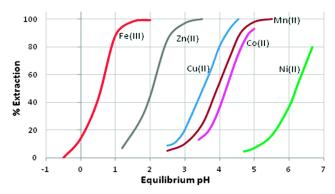
**Fig. 6** The pH-dependence of metal cation loading by Cyanex 272; data are adapted from <u>ref.</u> 22.
